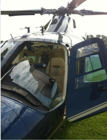
5th July 2011-A109C left windshield shattered by a Herring Gull (aw. 1.1kg/2.4lbs) impact. Pilot minor injuries. The co-pilot took control for an Emergency landing.
